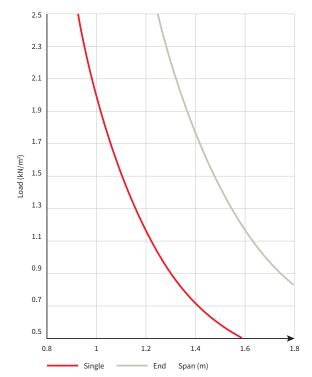
Safe span figures are based on a deflection limit of span/30 plus a safety factor of 1.2. It is assumed that the profile is crown fixed with at least six fixings at all purlins, including metal end laps onto the rooflight.
