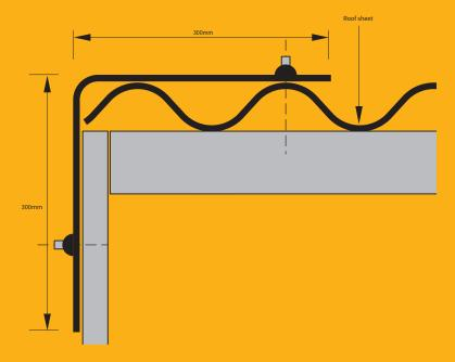
**Note:** As the verge is the part of the roof that is often the most vulnerable to wind damage, more fastenings are required there to ensure that bargeboards in general and the ends of the bargeboards are always securely fixed.
