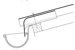
Note: The eaves closure pieces must not be used as an extension of the corrugated sheets.
