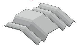
Where cranked crown sheets are used, it is especially important that the slopes are accurately aligned with each other.
