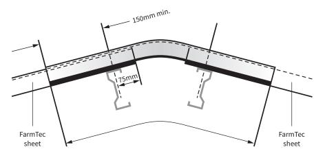
Fig 1 - Cranked crown and ventilated cranked crown fixings
