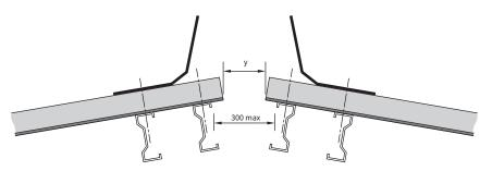
Fig. 1 Unprotected open ridge
