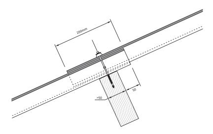
**Note:** When fixing to timber purlins, BS 5268: Structural use of Timber, recommends that the minimum edge distance of the fixing should be five times the fixing diameter to avoid undue splitting of the timber
