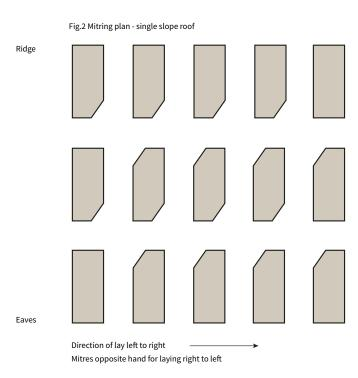
**Note:** All mass-produced building products are allowed certain dimensional tolerances. This applies to both profiled fibre cement sheets and steelwork. Because of these permitted variations in dimensions, regular checks should be carried out on measurements at mitres, and adjustments made as and when necessary.
