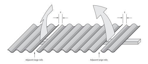
The benefits of using trimmed sheets in this way is that the sheets can be installed the right way up and have well-formed edge 'gutters' to prevent water dripping into the building
