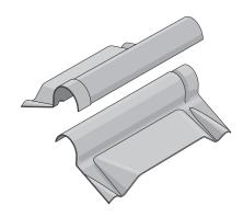
By using a plastic ventilation piece, the possibility of drifting snow and driving rain can be reduced but not eliminated. However, the reduction of the ventilation area provided decreases from 16200mm² to 12200mm².
