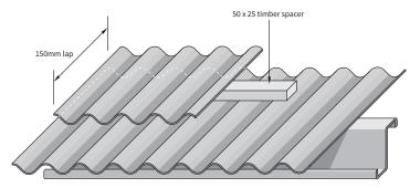
Fig. 3 Breathing roofs with battens
