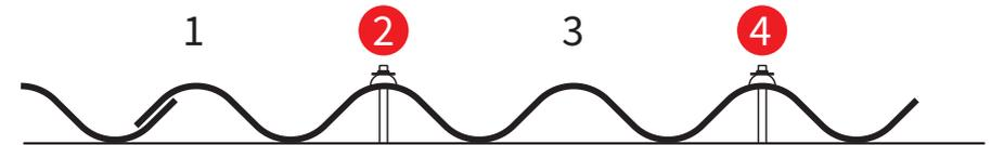
**Note:** Ensure when installing the outer roll, that the wings of the two piece ridges are sitting snug on the sheets and not pitched up or down.
