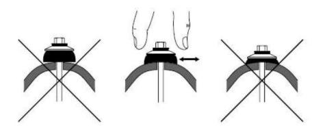
Fig. 4 Checking the topfix fasteners for tightness
