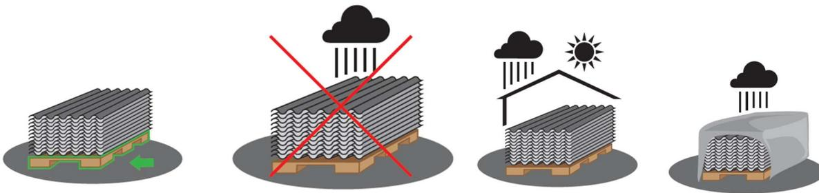
When the sheets are delivered, the packaging must be removed, the sheets must be left on the pallet and firmly stored on solid ground. Sheets cannot be stored in an open space, sheets should be placed under shelter, and if there is no possibility to do this, we recommend covering loosely with a weather resistant tarp to protect it against the weather elements.
